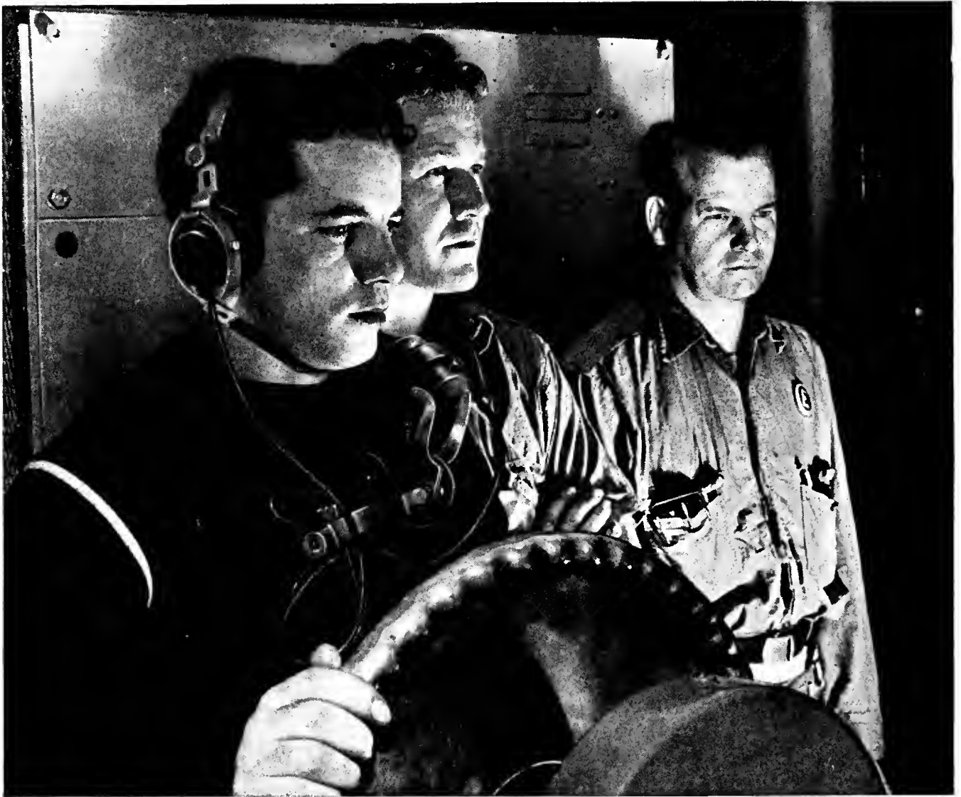
EMERGENCY STEERING STATION on U. S. battleship. The helmsman gets steering instructions over a battle telephone. The two other men are intently watching their gauges.
